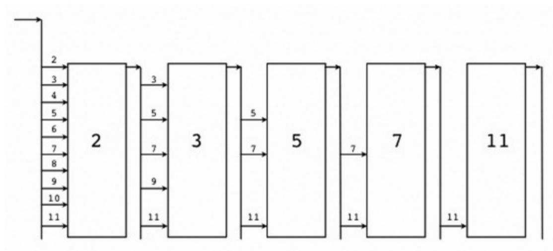
**Fig 14.2: The sieve prime-algorithm**
